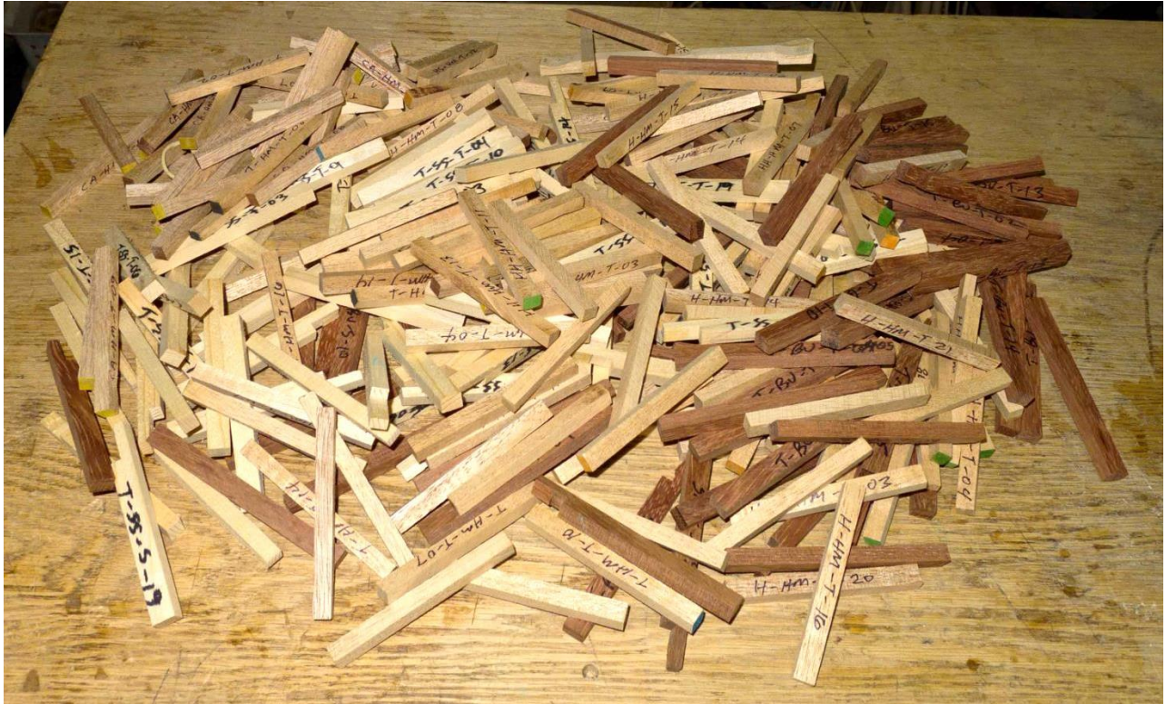
Figure 15: Pile of Failed Specimens Following Testing
