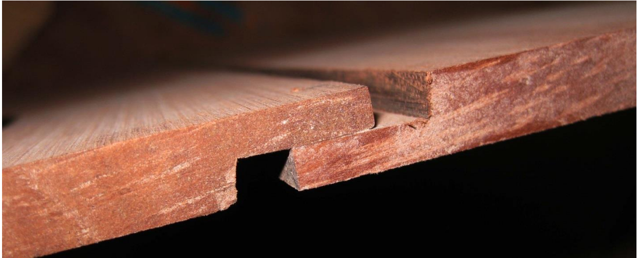
Figure 9: Detail of Shear Coupon Plate Glue Joint
